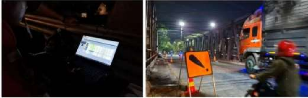
Gambar 5. Dynamic load test metode moving load traffic
